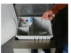
Remove the waste tank and empty.
