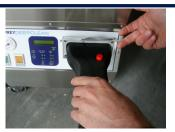
Open the front panel and connect the steam hose with the red button facing up. Push firmly and the hose will click into place
