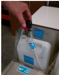
Remove black/red water reservoir cap and fill with clean cold tap water
