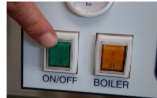
Plug machine into a suitable electric socket and press top section of green on/off switch
