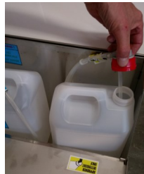
Fill grey/red cap chemical tank with manufacturers approved chemical if required*
