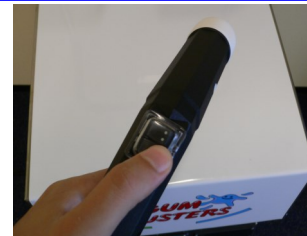
Plug machine into a suitable electric socket and press top section of green on/off switch
