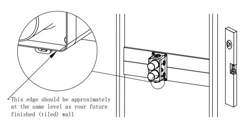
3. Use 1/2'' NPT fittings and thread seal tape for all pipe work according to the diagram below. No soldering close to the mixer body!
