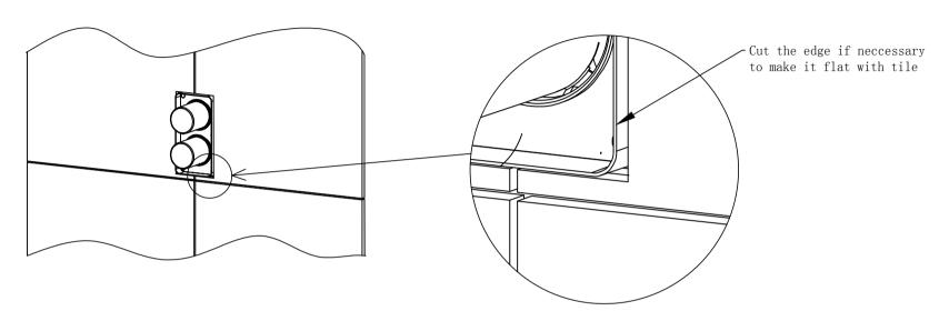
6. Remove protective caps. Install trim plate and handles.
