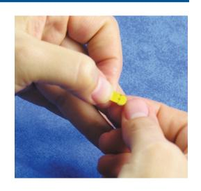
Step 1: Use the magnet end of the cleaning tool to pick up the battery on its flat side (the side with "+" sign).
