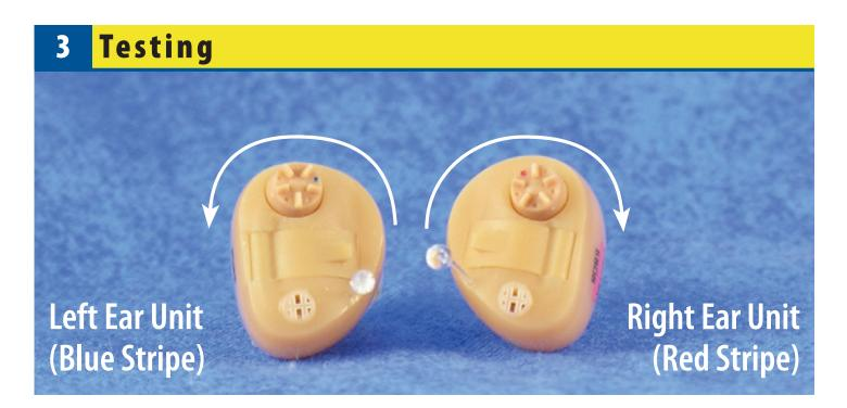
**Step 1:** With the volume wheel on top turn the volume wheel to full volume (counter clockwise on LEFT BLUE unit and clockwise on the RIGHT RED unit). If the device is in your ear, full volume is towards the front of your head for both units.
