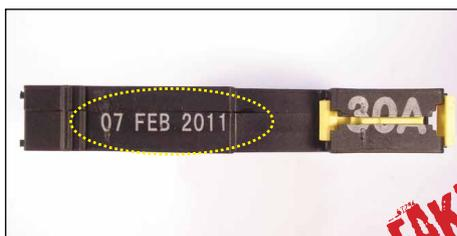
Date stamp on bottom of device. Imitation devices have a machine applied mark, whereas authentic devices have 100% quality inspection and the date stamp is applied by a quality inspector by hand.
