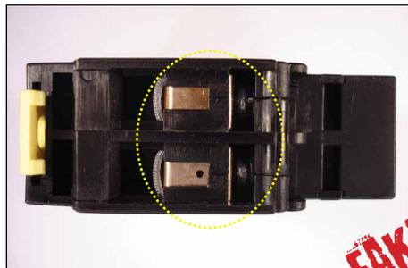
Imitation devices have one terminal with a locating hole, and one without. Both terminals on authentic devices have locating holes.
