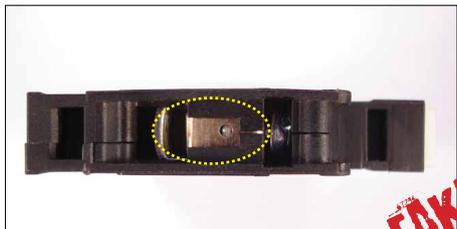
Imitation devices have holes in the terminals, authentic devices do not.
