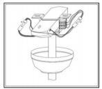
Make the wiring connection as shown in the picture. Ensure that the DIP switches on the receiver and transmitter are set to the same positions.
