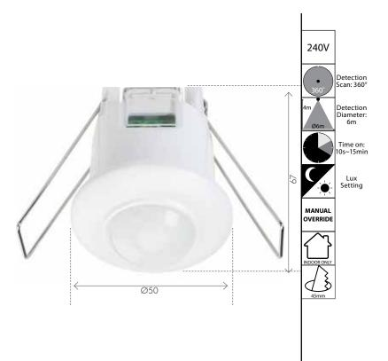
Passive Infra-red technology. Multi-segmented lens for better detection. Reliable 3-wire design. Adjustable time and lux level. Manual override Ceiling recessed mount Indoor use only. Resets to AUTO mode after 8 hours Lux control level : 3-2000LUX (adjustable) Max Load : 800W Incandescent Lamp 400W Fluorescent Lamp 200W LED Lamp
