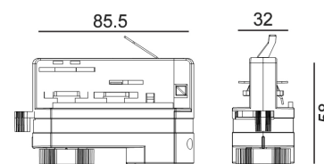
TRK3WHADAP3 TRACK 3 Circuit 4 Wire Adaptor Big Hold Weight 10Kg Max WH
