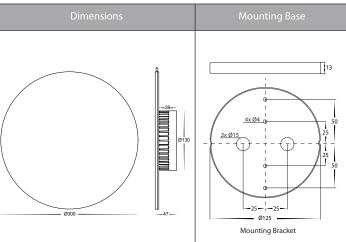
This fitting only requires a 2 core low voltage cable as RGBW Controller is installed internally into each fitting, Controller can also be removed and installed using any of our RGBW Controllers available though this will require a 5 core cable being run to each fitting.
