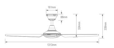
Note: Do NOT install on a raked or sloped ceiling without the use of the optional 38° Ceiling Kit, as this will damage the receiver housed in the canopy. \**If 38° ceiling kit is used the fan will no longer be IP66.*
