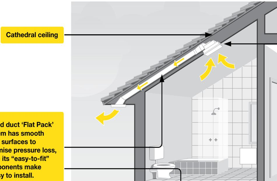
A rigid duct 'Flat Pack' system has smooth inner surfaces to minimise pressure loss, while its "easy-to-fit" components make it easy to install.
