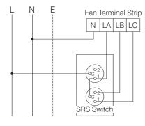
Note:-1. Remove link at fan terminal strip 2. Fan is double insulated - no earth required.
