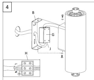
Connect supply cable to terminal block:
