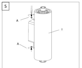
Slide fitting body 'I' onto mounting bracket 'B ' and tighten screws 'A' firmly.
