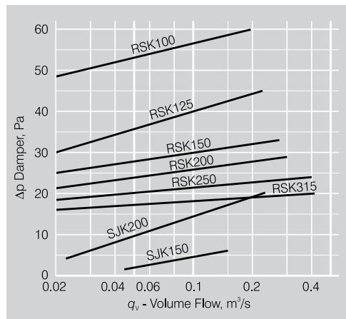
Compared to conventional spring loaded backdraft dampers, the SJK has superior performance characteristics due to its unique design that provides minimal resistance to air flow. The flap closes when the fan is off.
