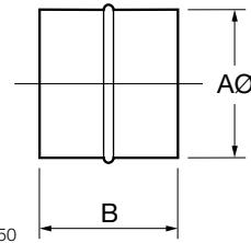
The tube is constructed from galvanised steel and the flaps from aluminium. Flaps are spring-loaded and when the fan is switched off they close providing a seal.
