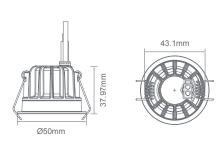
Ceiling cut-out Ø44mm / 3-25mm thickness
