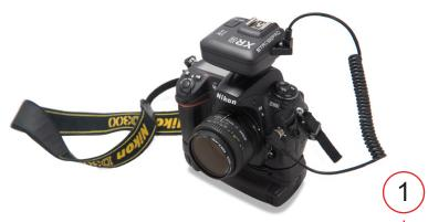
Connect the provided N1 or N3 Shutter Release cable to the XRN and camera port
