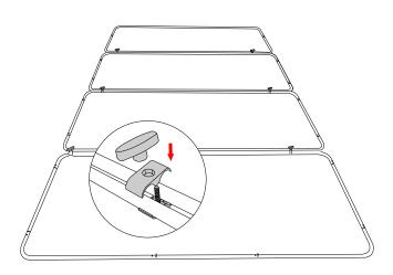
**3** Use hinge clips to connect two frames.
