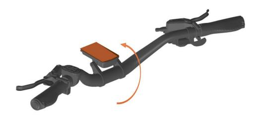
Place the handlebar at an appropriate position, and make sure the "cross symbol" is located at the center.
