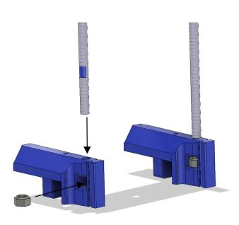
Start with getting the two locknuts inside each comportment, then screw the m8 metal rod until it's flush with bottom
