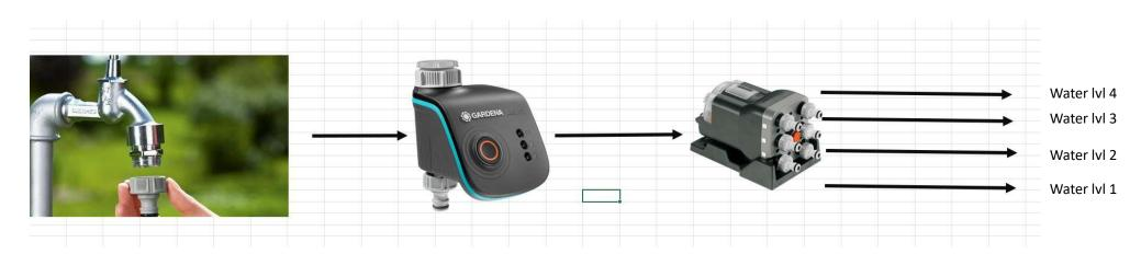
Use water directly from tap and connect to it to the smart controller. Then program it to the mechanical water distributer that works with pressure. When the pressure stops the mechanical water changes outlet so only 1 outlet is active. This works well if you have multiple levels.
