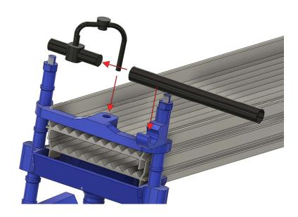
Make sure the 13mm tube goes all the way inside the connector.
