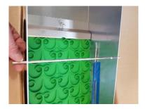
First place the m8x16mm bolt from inside the hopper facing outward and fit a nylon washer between the two aluminium surfaces (see below) and on the outside before fitting the flange nut.
