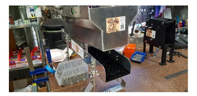
You will note each mount has three settings, this allows variation in hopper fall and tilt form the rear. Using the lowest setting here allows the full clearance of your hopper to rest inside the sluice channel.
