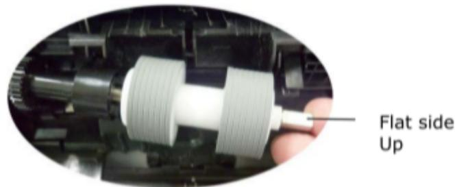
2. Insert the left end of the Reverse Roller to the hole of its original place.
