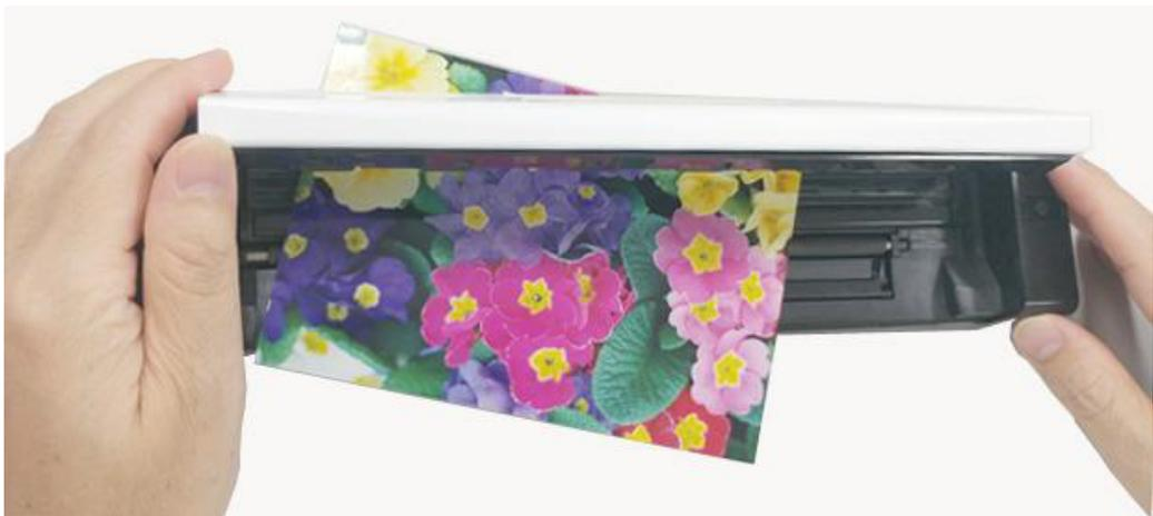
3. Close the cover and reinsert the item to rescan. The light will stop flashing once closed
