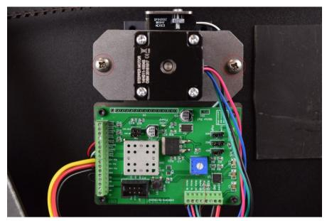
10. Connect the motor wires as shown on the wiring diagram
