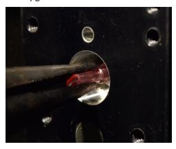
6. On the traverse board, release the wires from the push-in connector by pushing a pin or needle into the slot above the wire on the connector. Note which red and black wires go to the speed potentiometer input and which go to the power in. Terminals are labeled on the board opposite side of the connector. Some models used a red instead of white wire for the potentiometer as shown on the wiring diagram. Be sure not to swap a potentiometer wire with a power wire.
