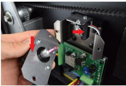
Make sure the urethane coupler slides onto the acme screw drive shaft and firmly push the motor towards the traverse board mount assembly until the motor mount plate is flat against the ears on the traverse board mount assembly. Use the included Philips screws and nuts to secure the motor mount plate to the traverse board mount assembly.
