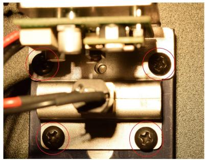
4. Pull the traverse board mount/bracket away from the traverse block. There will be some resistance as the urethane coupler separates from the acme drive shaft.
