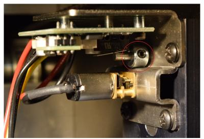
3. Remove the four screws securing the traverse motor/board mount bracket to the traverse block using a #2 Philips or 3/32" allen key
