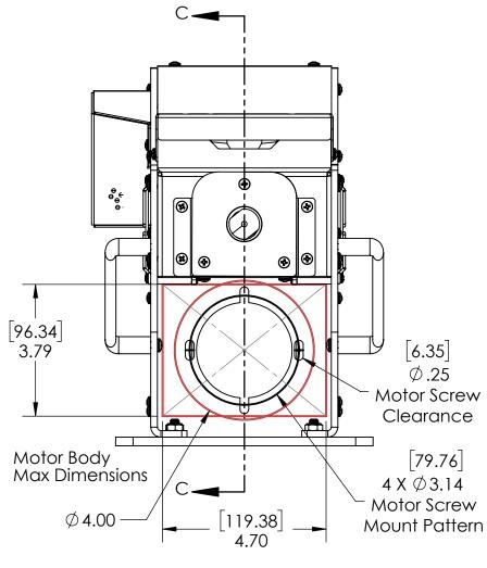
Drive Pulley Shaft Requirement: 22mm OD, 6mm Keyway
