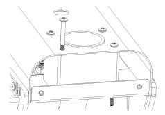
d. With the bolts removed, insert the supplied (4) cap head screws in from the bottom and thread them into the nylon lock nuts as shown in the picture below.
