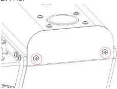
b. Swing down the front cover to expose the internal components.
