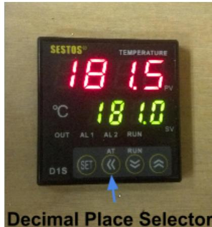
Step 5: Adjust the desired temperature using the “Up” and “Down” buttons.
