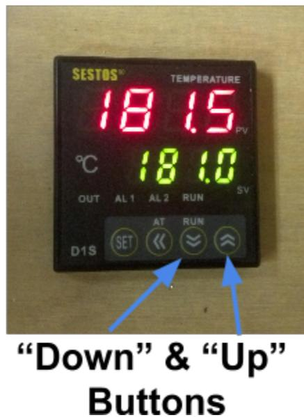
Step 6: Once desired temperature is set, press the “Set” button to lock it in. Pressing once will change the green numbers to a countdown of the relay, pressing it again will change to display of the desired temperature. Repeat process to change or lower temperature.
