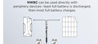
With additional cable, **NWBC** can be used with any Nett Warrior compatible power manager to scavenge and charge equipment efficiently.
