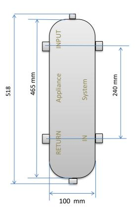
All sizes are supplied with insulation jacket - The top and bottom ports are typically for an AAV and Drain vale (supplied seperately)
