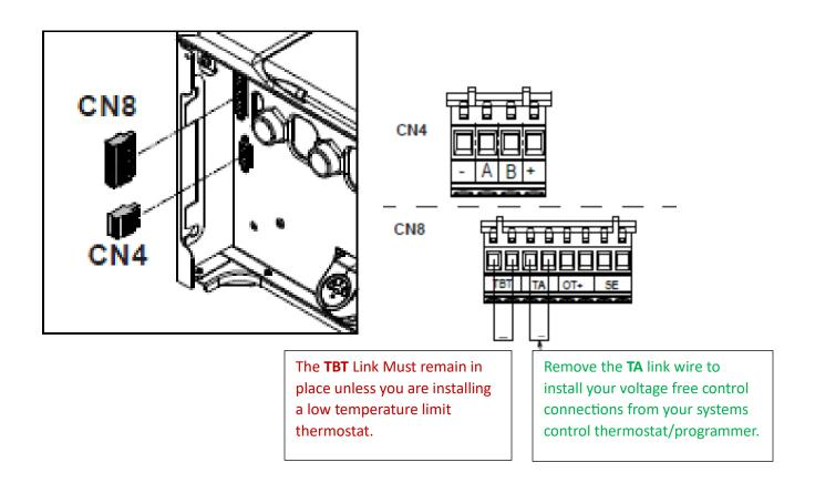
Ensure the connectors CN4 and CN8 are pushed fully home.
