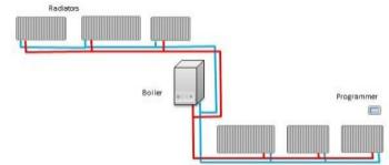
With a flow and return based system a single programmer is provided to control the on and off periods for the entire system , in some cases the system may be split to two flow and return circuits say upstairs and down, each with its own programmer.
