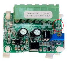
There are two subtly different formats of the Pump flow feedback board one with and one without the yellow jumper tag circled They are interchangable
