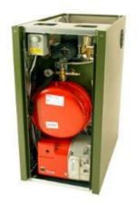
Models up to 120HE are supplied with System Kit SK1 having a capacity of 12 litres suitable for a maximum total system volume of 145 litres. Refer to BS7074 and the Boiler Manual for further guidance on expansion vessel sizing.
