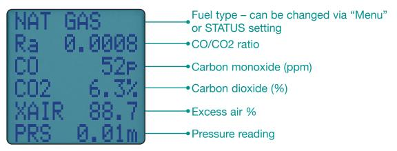
Press <a>> button to send a full combustion test to our optional KANE</a> IRP-2 printer or KANE's App via Wireless module.
