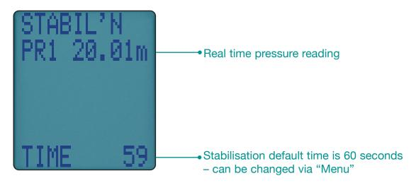
When complete press 🕶 to start the tightness test:
