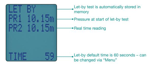
If let-by test fails rotate dial to another position to stop the test.
