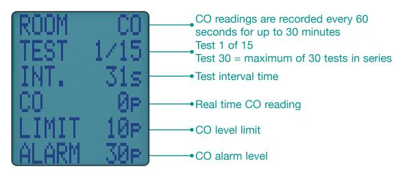
You can stop the Room CO test at any time by pressing  $\leftarrow$ .
