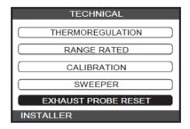
2/ Select CONFIRM to confirm the reset of the flue gas probe meter or else CANCEL to cancel the operation
