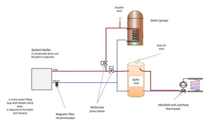
Mechanical Schematic (Gas or Diesel systems)
