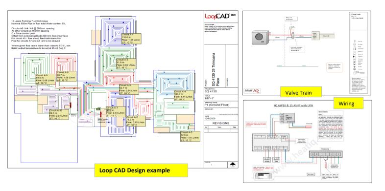
This detailed loop-CAD design will be accompanied by a mechanical valve train schematic and a detailed wiring diagram suitable for your electrical contractor to wire in for your system.
