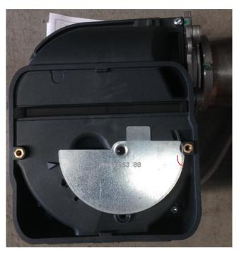
This one is the latest version with just a plain semicircle damper plate with no Adjustable positioning.
