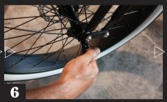
Insert and tighten front axle pin
