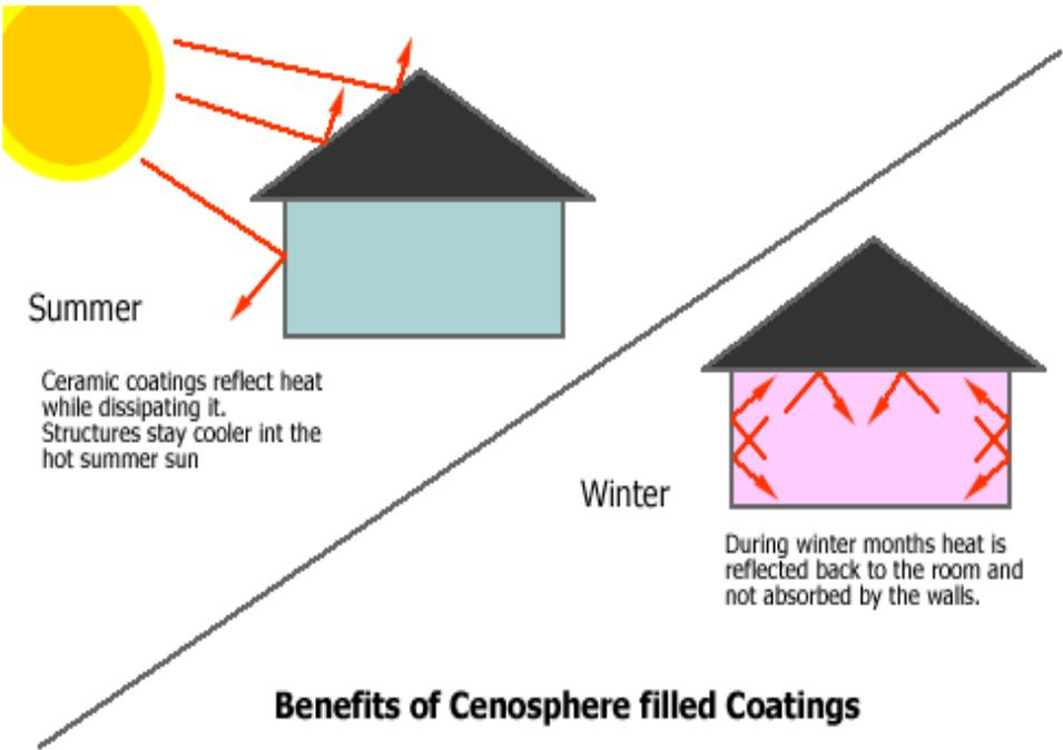
Ceramic microsphere coating systems can improve the energy efficiency of any structure by painting interior walls (outside) and ceilings to keep heat in during the winter and cool in during summer.
