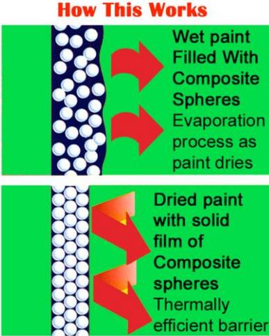
Rooms painted with hollow ceramic microsphere systems (ceiling and walls) will feel warmer at the same temperature than before the application. This is the same phenomenon as a person being outside in the sun and feeling hotter than being in the shade even though the temperature is the same. Further, walls painted with these coatings will be more durable as the ceramic microspheres create a hardened surface.
