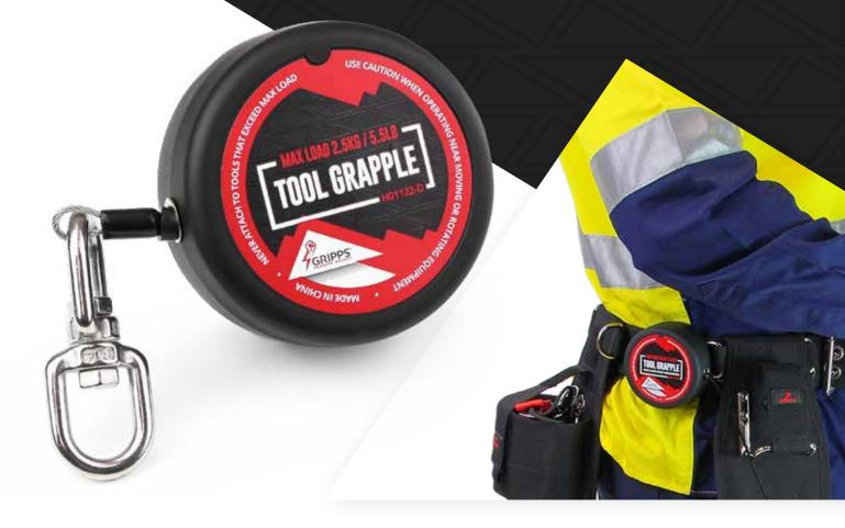
Able to be attached to a harness, work belt or wrist band, simply connect your tool to the Tool Grapple® via a GRIPPS® tool connector or tether. The wire tether automatically retracts and is available with an auto-stopping function that takes the tension out of the tether when the attached tool is in use. Dynamically tested for hand tools weighing up to 2.5kg/5.5lbs.
