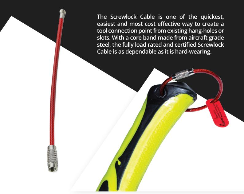
Create your secure tool connection point by simply threading the Screwlock Cable through an existing hanghole/ slot in your tool, and screw closed. Add a drop of thread-locking compound before you screw shut to create a permanent, load rated connection point on your tools.
