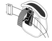
To anchor Bolt-Safe Pouch to a harness, loop the velcro strap around the harness and through the plastic buckle.
