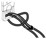
Feed the carabiner end of the tether through the loop and pull tightly to create a secure connection.
