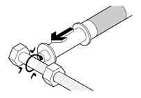
Slide the wire noose over your bolt/nut and slide up till reaching the top of your screw is reached. Release the shaft to secure it tightly.
