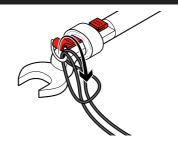
To attach using the loop end, pass the loop through a connector point.
