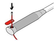
Feed the Screwlock Cable through the pre-formed hole in the tool.
