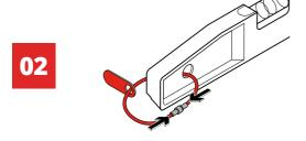
Join the two ends together, ensuring a firm application and click sound is heard/felt. Test Gripplock Cable cannot be separated by tugging both ends firmly.
