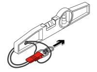
Feed the Swivel Catch cord through the pre-formed hole in the tool
