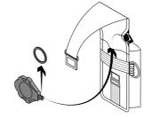
Remove Tool Ring from retractor then insert the Retractor Unit into back pouch.
