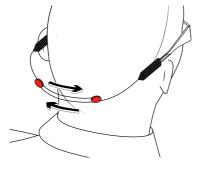
Place eye wear and Safety Glasses Tether on head. Adjust the Safety Glasses Tether by sliding the two red central pieces to opposite sides.
