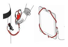
Apply the clip of the coil tether to your clothing by sliding the clip over the garment and snapping shut the clip. Ensure the clip is closed correctly by testing, firmly pull-on tether to check for a secure hold.
