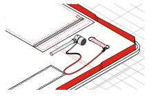
Ensure that tools are tethered to one of the 8 D-Ring anchor points on the Modular Drop Mat when working at height.
