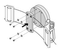
Place harness or belt on Tool Grapple then screw the belt cover back on. Ensure the position of the Tool Grapple® does not interfere with the functionality of the harness.
