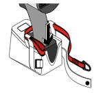
Insert the battery pack (whilst connected to the power tool) into the Battery Catch Holster.
