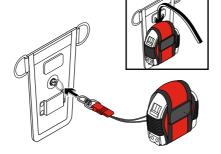
The Tape Measure Catch can now slide onto the Tape Measure Latch.
