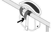
To anchor Bolt-Safe Pouch or Rail Bag to a rail, pass the velcro strap around the rail and through the buckle, pulling tight.
