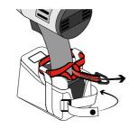
Secure the holster by pulling the strap tight and click in to the closest button. Ensuring the choke strap passes through the three choke guides, pass the D-Ring end through the loop end of the choke.
