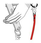
Once the tool ring is applied to your chosen tool, connect the tool ring to a GRIPPS® tether of choice.
