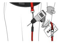
Attach a GRIPPS® tether with an appropriate load rating to the D-Ring on the choke strap.
