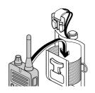
To secure an electronic device, slide the radio or device all the way to the bottom of the holster.
