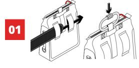
For applying to a work belt, feed work belt through rear loops and then secure belt to your waistline. Alternatively attach a carabiner to top loop, threading carabiner through and secure carabiner for harness work
