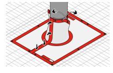
Ensure the fastener strip is firmly pressed all the way along from top to bottom. Fasten all eyelets around piping with suitable ties.
