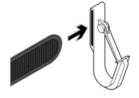
Thread work belt through the loop of Battery Operated Arrest Holster.
