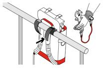
To secure to a rail, wrap the straps all the way around the rail and feed back through the metal bracket.
