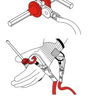
Two Little Grippers may be used without a GrippLink when using GRIPPS H01067 tether.
