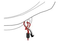
Feed the looped end of the hard hat tether through an appropriate connector point on the hard hat.
