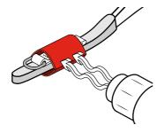
Apply a heat gun to the Gripp Shrink. Use the heat gun evenly and rotate the tool continually whilst applying heat. Allow to cool.
