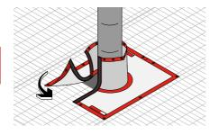
Surround pipe with Gap Wrap. Overlap central Velcro fasteners strips.
