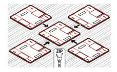
To connect multiple Modular Drop Mats together, align zips on both Modular Drop Mats and zip end-to-end.
