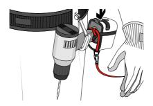
Your tethered drill (or similar device) can be stowed into the BOA after by simply pressing your tool into the latch. The latch utilizes a spring to automatically lock after. To remove your tool, press latch inwards and pull tool out. Ensure your tool is properly anchored before using BOA holster
