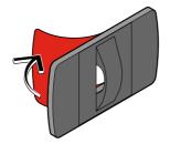
Peel cover from one side of the adhesive pad and attach to the E-Catch. Peel cover from other side and attach to a non-porous location on the device.
