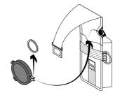
Remove tool ring from Retractor then insert retractor into holster pocket. Feed end of retractor cable out of holster pocket.
