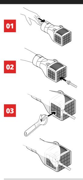
Place hand inside Bolt-Vault, firmly strapping around the wrist by feeding the strap through the buckle and pulling tight.
