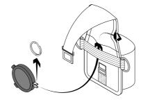
Remove Tool Ring from retractor then insert the Retractor Unit into back pouch, then reattach tool ring.
