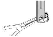
Using the needle nose pliers, thread the pried-open halves of the Tool Ring into the tool aperture.
