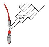
Squeeze a drop of threadlocking compound onto the cable thread for a permanent connection point.
