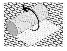
Place roll of GRIPPGrid on gridmesh floor in desired location. Roll out matting ensuring material is flat without kinks.
