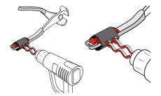
Slide Gripp Shrink over Tool Catch and V-Gripp Tape. Then apply heat gun over V-Gripp Tape, covering all areas until fitted securely.v
