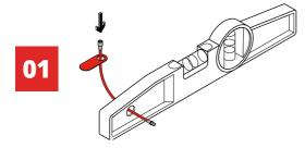
Feed the Gripplock Cable through the pre-formed hole in the tool.
