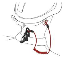
Push fabric all the way into the jaws of the clamp, ensuring that the clamp 'teeth' are totally covered by fabric.
