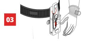
Your Gripplock Cable is now ready to connect with a suitable GRIPPS® tether.
