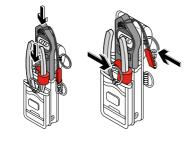
Connect tool to the Retractor or side D-Rings.
