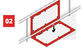
For use on gridmesh flooring, lie Gap Mat flat and apply ties to eyelets.
