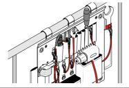
When you no longer need the tool, place back into the GTS pouch, reattaching the tether to an anchor point.
