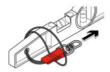
Feed the Swivel Catch through the pre-formed hole in the tool. Loop Swivel Catch back through itself. Your tool is now ready to connect to a GRIPPS® Retractable Tool Belt via a GRIPPS® Retractor Unit.
