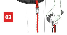
Your Tool Hitch is ready to be tethered to a suitable anchor point using an appropriate GRIPPS® Tool Tether.
