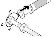
Compact the Bolt Gripper shaft downwards by firmly pressing your fingers on the shaft; expanding the opening.
