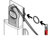
Reattach tool ring to Retractor end.
