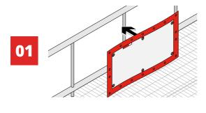
For handrail use, place Gap Mat against handrail and apply ties to eyelets. Ensure Gap Mat is flush with floor.
