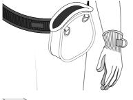
Then pull the strap tightly and press firmly together to attach.
