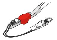
The D-Ring of your Tool Catch is now ready to connect with a suitable GRIPPS tether or Swivel Catch.
