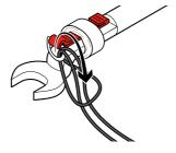
To attach using the loop, pass the loop through a connector point on the tool.
