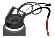
Connect an appropriate GRIPPS ® tether to the top of the bottle on the attachment point.
