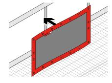
Place Gap Screen against handrail and apply ties to eyelets. Ensure Gap Mat is flush with floor.
