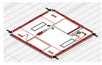
To secure the Modular Drop Mat, use cable ties to secure all of the eyelets to the workplace.
