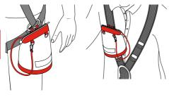
Connect the carabiner to an appropriate anchor point on the harness.
