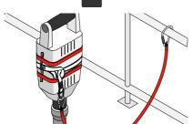
Your Tool Hitch is ready to tether to a suitable anchor point using an appropriate Tool Tether.
