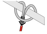
For SKU H01076 - Feed the carabiner end of the tether through the loop and pull tightly to create a secure connection.
