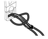
Connect a GRIPPS tool tether with a loop ending, (e.g. H01073) by passing the loop end of tether through the enclosed bottom hole of carabiner. Weave the tether back through it's own loop to create a choke-hold. Pull tight to secure
