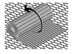
Place roll of GrippAir on gridmesh floor in desired location. Roll out matting and cover length of desired area. Ensure matting is flat without raised bubbled spots.
