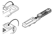
Open top cover. Slide Radman all the way to the bottom of the holster. Close top cover after.
