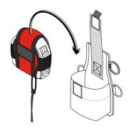
Attach Swivel Catch to the Retractor Unit D-Ring. Slide holster onto work belt and situate on belt as desired.
