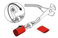
Slide Gripp Shrink over Tool Catch and V-Gripp Tape, ensuring the D-ring is left exposed and accessible.
