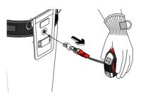
Attach holster to your work belt by sliding belt through the rear straps of the Tape Measure Latch Holster.
