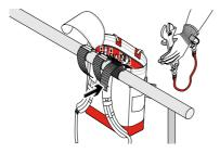
To secure to a rail, wrap the velcro mounting straps all the way around the rail and feed back through the metal brackets. Adhere velcro strap.
