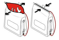
To operate the metal-snap mechanism, pull the opening apart and the closure will automatically spring open and lock into place.
