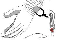
If using the poly single-action model, anchor the tether on the load-rated anchor point on the back of a GRIPPS® glove.
