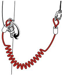
If anchoring to clothing, ensure you clip the tether onto thick fabric such as your collar or pocket lining.
