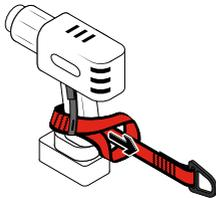
Pass one end of the Tool Hitch around the neck (near tool's center of gravity). Then pass the D-Ring end back through the Tool Hitch loop to create a choke-hold.
