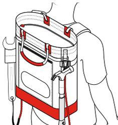
To manually transport, use backpack straps, and adjust length as required. Refer to your workplace guidance on safe manual handling guidelines.
