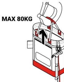
To lift, zip the lid closed to secure contents. Ensure all tools are tethered to D-Rings. Attach lifting hook to both of the lifting straps.
