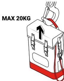
To lift, clip the lid closed to secure contents. Ensure all tools are tethered to D-Rings. Attach lifting hook to the red upper lifting strap.
