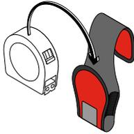
Insert Tape Measure into GRIPPS® Tape Measure Catch.
