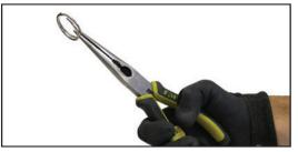
2. Using the needle nose pliers, thread the pried-open halves of the Tool Ring into the tool aperture.
