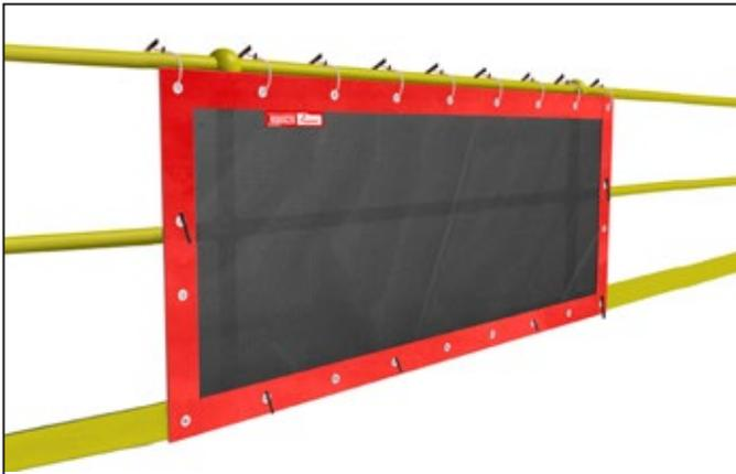
The GRIPPS Gap Screen is an economic fire-resistant drop prevention barrier for handrails. The Gap Screen allows personnel to work on platforms at height whilst protecting their tools and equipment from rolling off platform edges. The Gap Screen is secured using cable ties (or similar) via the 22 available stainless steel eyelets.
