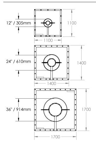
The GRIPPS Gap Wrap is a unique encapsulation device, designed to eliminate the gap found around pipes that run vertically through jobsite flooring.
