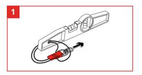
Feed the Swivel Catch cord through the pre-formed hole in the tool.
