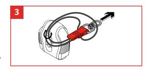
Apply the Swivel Catch, by choking it through the D-Ring.
