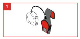
Insert Tape Measure into GRIPPS® Tape Measure Catch.
