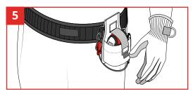
Your measuring tape is now ready to be applied to a GRIPPS® Retractable Tool Belt or other suitable GRIPPS® tether.
