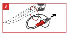
Apply the Swivel Catch, by choking it through the Screw Lock cable.
