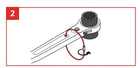
Apply a small amount of thread locking compound to the inner thread. Then screw ends of cable together completely.
