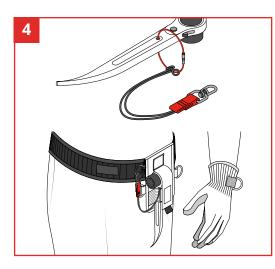
Your Ratchet/Wrench is ready to apply to a GRIPPS® Retractable Tool Belt or other suitable GRIPPS® tether.
